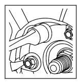
3. Using the wheel wrench, loosen all the wheel nuts by turning the nuts one turn counterclockwise. Do not remove them yet.
