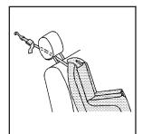
For vehicles that have a headrest or head restraint, fold down the headrest or head restraint and route the single tether under the headrest or head restraint and in between the headrest or head restraint posts.
