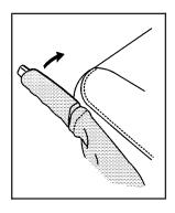
To set the parking brake, hold the regular brake pedal down with your foot and pull up on the parking brake lever located between the seats. If the ignition is on, the brake system warning light on the instrument panel cluster will come on. See *Brake System Warning Light on page 3-36*.
