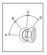
The ignition switch has four different positions.
