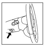
The tilt lever is on the outboard side of the steering column, under the turn signal lever.
