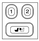
If your vehicle has this feature, the controls for the memory function are located on the driver door.
