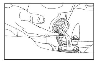
3. Fill the radiator with the proper DEX-COOL coolant mixture, up to the base of the filler neck. See *Engine Coolant on page 5-29* for more information about the proper coolant mixture.
