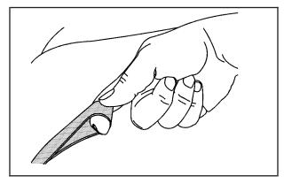
Pull up on the loop located where the seat cushion meets the seatback and flip the seat cushion forward. *Notice:* Folding a rear seat with the safety belts still fastened may cause damage to the seat or the safety belts. Always unbuckle the safety belts and return them to their normal stowed position before folding a rear seat.
