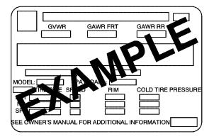
A vehicle specific Certification/Tire label is found on the rear edge of the driver's door. The label shows the size of your vehicle's original tires and the inflation pressures needed to obtain the gross weight capacity of your vehicle. This is called Gross Vehicle Weight Rating (GVWR). The GVWR includes the weight of the vehicle, all occupants, fuel, cargo, and trailer tongue weight, if pulling a trailer.
