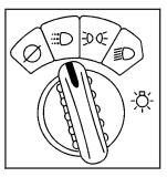
The exterior lamps knob is located on the instrument panel.
