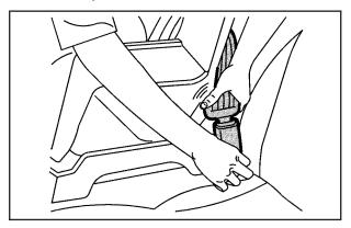
Push the latch plate into the buckle until it clicks. Position the release button on the buckle so that the safety belt could be quickly unbuckled if necessary.
