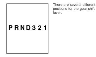
**P (Park):** This position locks the rear wheels. It is the best position to use when you start the engine because the vehicle cannot move easily.
