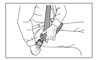
3. Push the latch plate into the buckle until it clicks. Pull up on the latch plate to make sure it is secure. If the belt is not long enough, see *Safety Belt Extender on page 1-32*.
