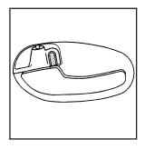
You can lock or unlock the door from the inside by sliding the manual lever forward or rearward.
