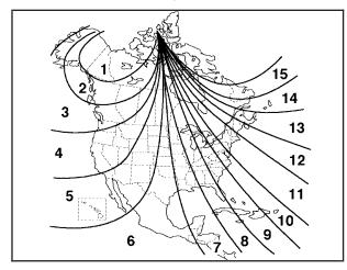
Press and hold <sup>()</sup> or depending on the mirror, press COMP until a Z and/or a zone number displays. The compass is now in zone mode.
