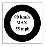
16. If the flat tire was able to inflate to the recommended inflation pressure, remove the maximum speed label from the sealant canister (E) and place it in a highly visible location.
