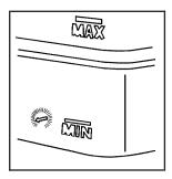
The fluid level should be above MIN. If it is not, have the brake hydraulic system checked to see if there is a leak.
