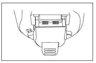
The vehicle may have a seven-wire trailer towing harness. This harness may have a seven-pin universal heavy-duty trailer connector (if equipped with the trailering package) that is attached to a bracket on the hitch platform or included with the four-pin trailer towing harness. If the vehicle is not equipped with the heavy-duty trailer connector, one may be purchased from your dealer/retailer. The seven-wire harness contains the following trailer circuits:
