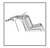
If the position you are using does not have a headrest or head restraint and you are using a dual tether, route the tether over the seatback.
