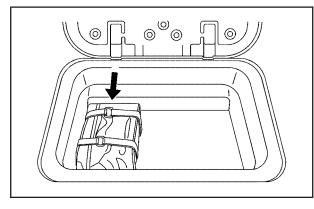
The tire sealant and compressor kit is attached to the floor with two straps.
