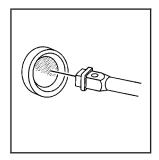
Insert the socket end of the extension (C) on a 45 degree angle downward into the hoist drive shaft hole.
