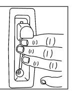
2. Lift the lever, located on the outboard side of the seatback, and fold the seatback forward.
