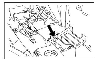
The jacking equipment needed to remove the spare tire is stored under the rear seat. To release the jack from its holder, turn the knob on the jack counterclockwise to lower the jack head. See *Rear Seat Operation on page 1-11* for more information. The tools you will be using include:
