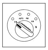
Use this knob to shift into and out of four-wheel drive.
