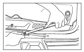
Turn the wheel wrench counterclockwise to lower the spare the rest of the way.
