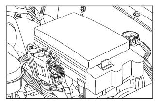
The fuse block is located under the hood in the engine compartment on the driver side of the vehicle. See *Engine Compartment Overview on page 5-12* for more information on location.
