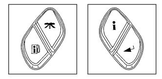
**(Trip Information):** Press this button to display the odometer, trip odometers, tire pressure, and timer.
