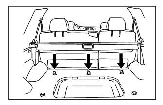
The top tether anchors for each rear seating position are located on the floor in the cargo area of your vehicle. Do not use the rear tie-down brackets near the liftgate for attaching top tethers. Be sure to use an anchor located on the same side of the vehicle as the seating position where the child restraint will be placed.
