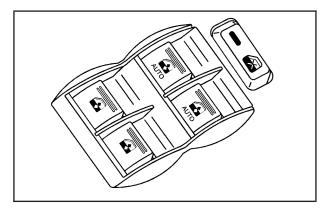
The controls for the power windows are located on the armrest on each of the side doors. With power windows, the switches operate the windows when the ignition is in ON/RUN, ACC/ACCESSORY or when Retained Accessory Power (RAP) is active. See *Retained Accessory Power (RAP) on page 2-23*. The driver's door also has a switch for each of the passenger's windows.
