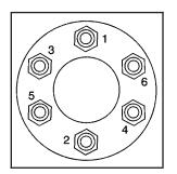
14. Use the wrench to tighten the wheel nuts firmly in a crisscross sequence as shown.
