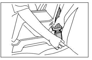
Push the latch plate into the buckle until it clicks. Position the release button on the buckle so that the safety belt could be quickly unbuckled if necessary.
