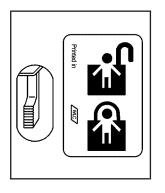
2. Move the lever down to engage the security lock. Move the lever up to disengage the security lock. The rear doors of your vehicle cannot be opened from the inside while this feature is in use. If you want to open the rear door while the security lock is on, unlock the door and open the door from the outside.
