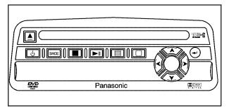
$\bigcirc$  (Power): Press to turn the RSE system on and off. The power indicator light illuminates when the power is on.
