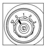
The rear wiper/washer button is located to the right of the steering wheel on the instrument panel. To turn the rear wiper on, turn the control to either 1, 2, or 3. For delayed wiping, turn the control to 1 or 2. For steady wiping, turn the control to 3. To turn the wiper off, turn the control to 0.
