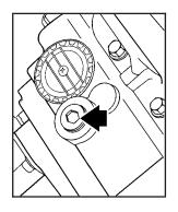
To get an accurate reading, the vehicle should be on a level surface. If the level is below the bottom of the filler plug hole, you will need to add some lubricant. Add enough lubricant to raise the level to the bottom of the filler plug hole. Use care not to overtighten the plug.
