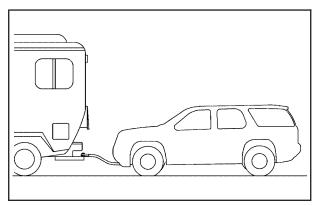
Four-wheel-drive vehicles can be dinghy towed if the proper procedures are followed. The transmission has no provisions for internal lubrication while being towed, so it is important that all the steps listed in this manual are followed to dinghy tow a four-wheel-drive vehicle. Use the following procedure to dinghy tow a four-wheel-drive vehicle:
