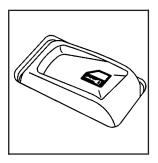
The power door lock switches are located on the driver's and front passenger's door armrests.
