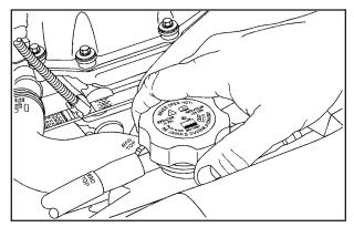
1. You can remove the radiator pressure cap when the cooling system, including the radiator pressure cap and upper radiator hose, is no longer hot.
