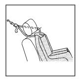
If the position you are using has a headrest or head restraint and you are using a dual tether, route the tether around the headrest or head restraint.
