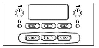
$\bigcirc$  (Power): Press to turn the system on or off. The rear speakers are muted when the power is turned on.
