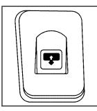
Press and release the back of the control in the overhead console to open the sunroof. Press the front of the control to close the sunroof.
