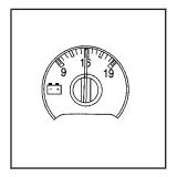
When your engine is not running, but the ignition is on, this gage displays the battery voltage in DC volts.
