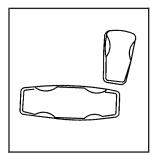
On vehicles with power seats, the controls used to operate them are located on the outboard side of the seats.
