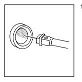
If the spare tire is hanging from the cable, insert the socket end of the extension into the hoist shaft hole on a 45 degree angle downward.
