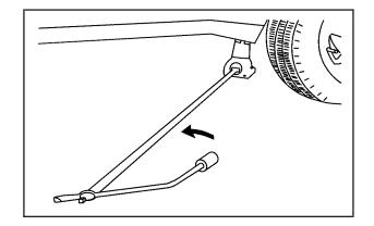
13. Lower the vehicle by turning the jack handle counterclockwise. Lower the jack completely.
